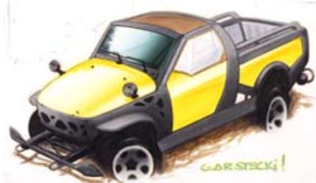
Trucks may become smaller, more compact and boast more functionality. This truck shows an exposed exoskeletal system, which is usually concealed but is designed to enhance safety and absorb more energy in a crash, creating another level of protection for passengers.
