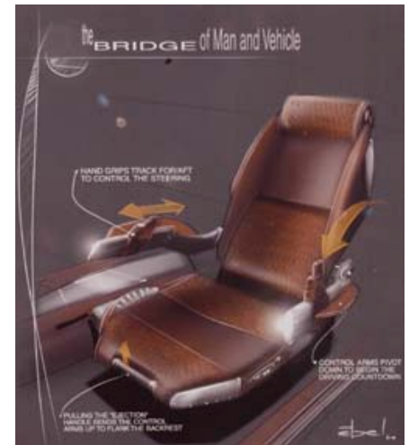
In the future, steering could be conducted by controls on the seat and not a steering wheel. Unitized seats may be more ergonomically appealing for drivers. Hand grips track backward and forward to control steering. Control arms pivot down to begin the driving countdown. An ejection handle located at the front of the seat sends control arms up to flank the backrest.
